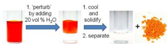
Figure 2. Polywax, THF, and DMF at 80 °C form a solution with the dye 1. Subsequent perturbation of this solution produces a biphasic mixture consisting of a Polywax phase and a THF/DMF phase. This nonpolar soluble polymer-bound dye (as well as fluorophore 2) partitions completely into the hydrocarbon phase which solidifies on cooling. Separation and drying leads to a 1/Polywax mixture which redissolves in THF on heating.
